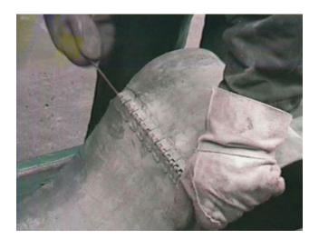
Now, in the same way add additional sections of belt. As the belt is lengthened, feed one end of it around the large roller on the belt-tensioning assembly and under the trays as shown in the left hand picture below.
